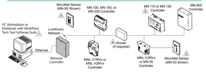
1 Programming any of the MicroNet LON controllers, or the TAC I/A Series MN 800 controller, requires WorkPlace Tech Tool (WP Tech).
